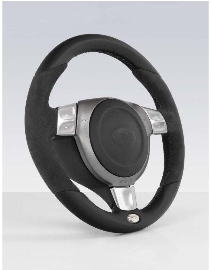
TECHART 3-Speichen Sportlenkrad Typ 2 in Alcantara TECHART 3-spokes sport steering wheel Type 2 in Alcantara
